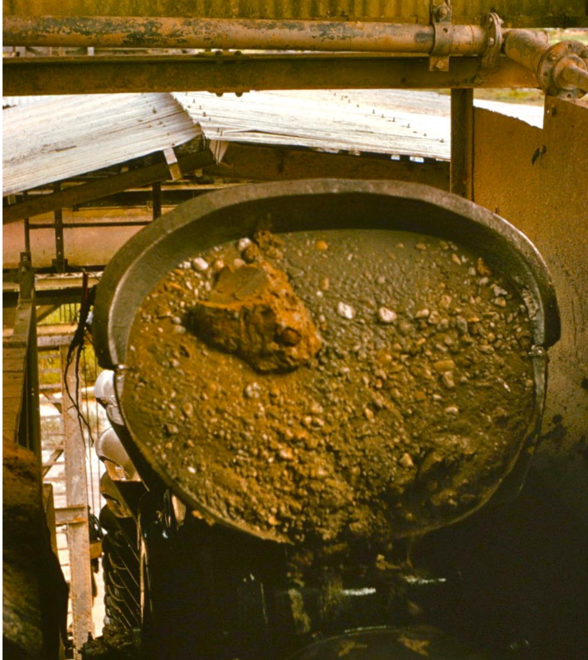
Figure 7. Steel scoop containing gravels excavated from Offin River Valley by Bremang Gold Dredge is lifted onto dredge during 1963 operations
